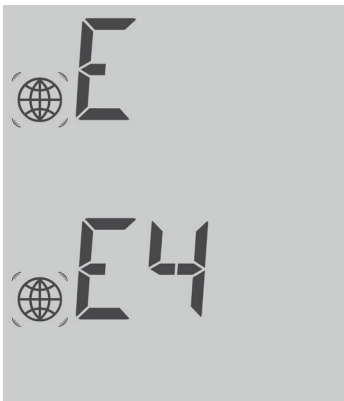
Fig.: Example for a blinking code sequence for Internet - Fault 4
