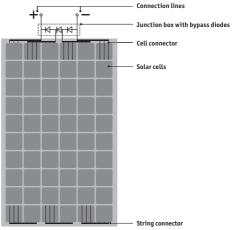
Module schematic, front view
