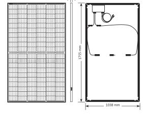
The dimensions and weight displayed in this table apply to modules manufactured from February 2021 (SPVxxx-R60DBMG-2M2C01). Modules manufactured prior to February 2021 (SPVxxx-R60DBMG-2C01) have dimensions of 1776 x 1052 x 40 mm and weigh 23.0 kg
