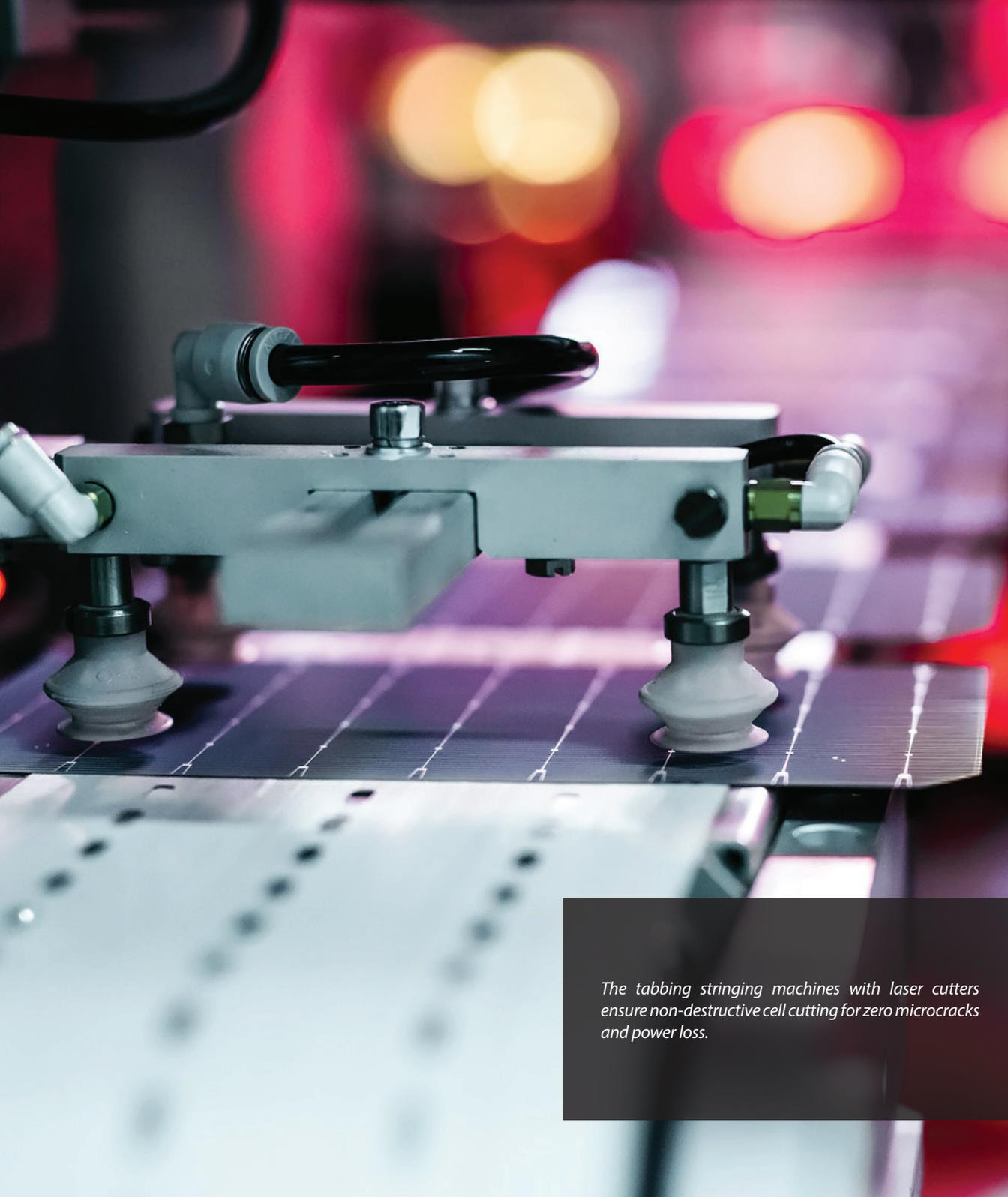
*The tabbing stringing machines with laser cutters ensure non-destructive cell cutting for zero microcracks and power loss.*
