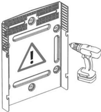
Figure 2.10 Mounting of the wall mounting bracket
