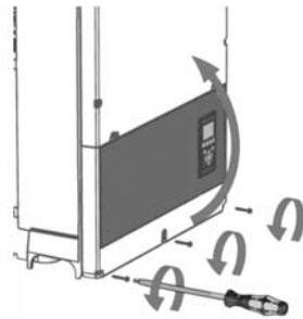
Figure 2.15 Loosen front screws and lift the cover
