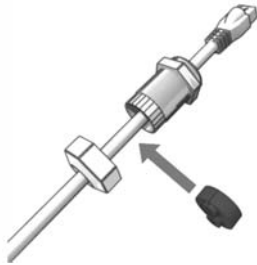
Figure 2.22 Run cables through cable glands
