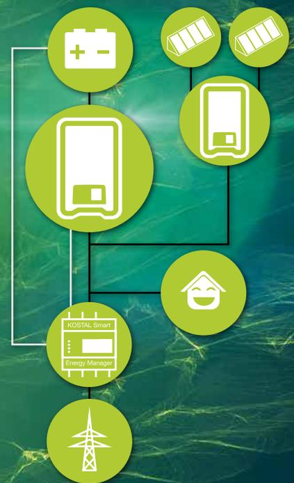
The PIKO MP plus can also be connected to an existing PV system on the AC side only, where it is used to store energy.
