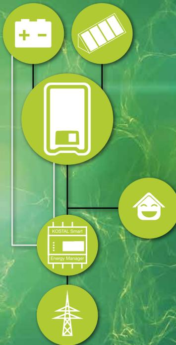
The KOSTAL Smart Energy Manager can be used to connect a battery and therefore store energy.
