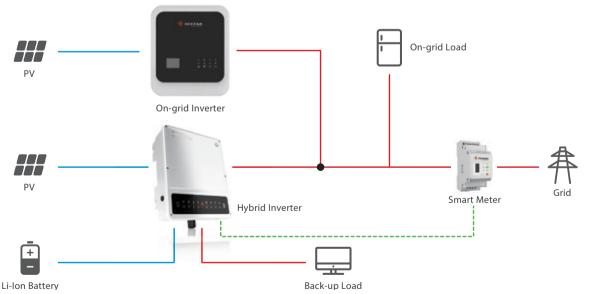
This solution integrates both hybrid and retrofit functions into a single system. In both on-grid systems as well as hybrids, the solar energy is used to supply electricity to both back-up loads and to charge the battery before the power is injected into the grid. By adopting such a solution, the system provides a more reliable source of supply for the loads, while ensuring a sufficient supply of green energy to charge the battery.
