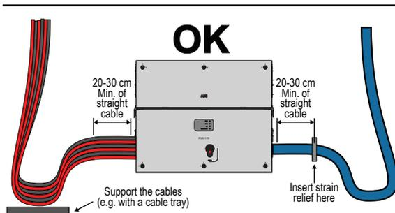
The AC and DC conductors must be anchored or supported in order to prevent loading and mechanical stress on the cable glands and quick fit connectors causing potential damage on the AC and the DC plates.
