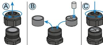
As an alternative the standard gasket of the cable gland can be replaced with the two-hole gasket. The two-hole gasket accepts two cables with a diameter of 6mm; if a seal hole is not to be used, it is necessary to install a plug (supplied plastic cylinder) to ensure the inverter's sealing.
