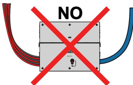
The cable routing have to be done in order to avoid water dripping to the AC panel cable glands **(11)** **(12)**, DC input quick fit connectors **(17)** or to service cable glands **(13)**.
