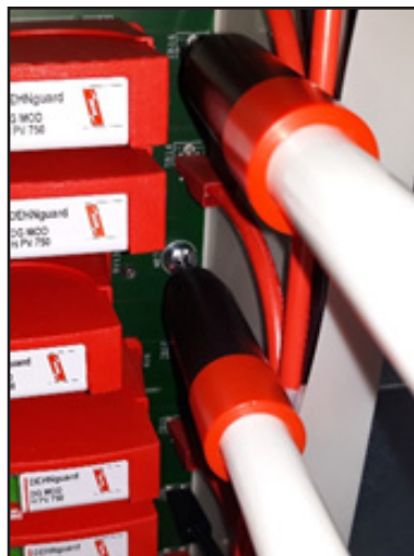
Example: VAT between CH9(-) and PE
