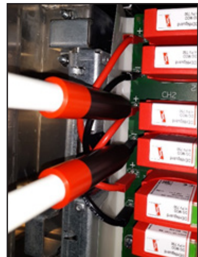
Example: VAT between CH2(+) and CH2(-)
